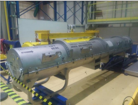
FIGURE 4: AMERICAN FRESH FUEL CASK
